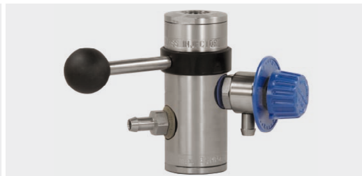
☞ 1/2" F - ☜ 1/2" F. Injector ST-168 with metering valve ST-161 and compressed air modul (hose tail 9 mm). Max. 350 bar / 100 °C
