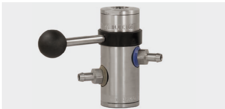
☞ 1/2" F - ☜ 1/2" F. Injector ST-168 with hose tail 9 mm and compressed air modul (hose tail 9 mm). The chemical dosing is adjusted by 8 exchangeable nozzle inserts (0.5 - 2 mm). Max. 350 bar / 100 °C
